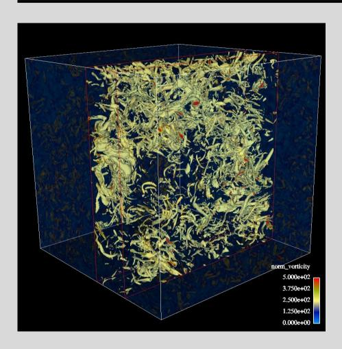
Vorticity iso-surfaces in a  $512^3$ sub-domain of the LANL decaying  $2048^3$  NS-simulation at  $Re_{\lambda} \sim 200$ . Uneven clustering results in intermittency; Batchelor & Townsend (1949); Kuo & Corrsin (1971), Sreenivasan & Meneveau (1988, 1991); Frisch (1995): courtesy of Darryl Holm.
