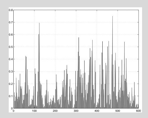
Dissipation-range intermittency from wind tunnel turbulence where hot wire anemometry has been used to measure the longitudinal velocity derivative at a single point (D. Hurst & J. C. Vassilicos). The horizontal axis spans 8 integral time scales with  $Re_{\lambda} \sim 200$ .
