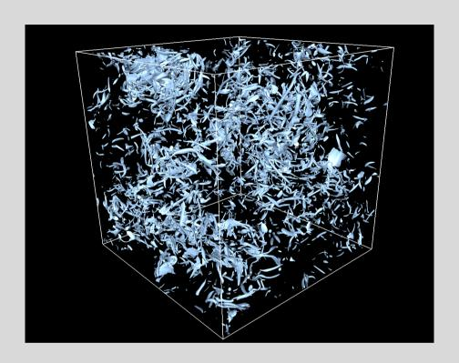
A 3D statistically stationary homogeneous isotropic NS-flow at  $Re_{\lambda} \sim 107$  showing isosurfaces of  $\omega^2$  at  $10 \times \omega_{av}^2$  in a  $(2\pi)^3$  cube resolved with  $2048^3$  points: courtesy of Jörg Schumacher of TU Ilmenau.
