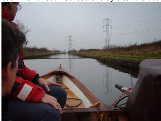
Whilst the engine created significant wash, the smooth soliton created by the boat can be seen well ahead. It arose shortly after the boat achieved the correct speed.
