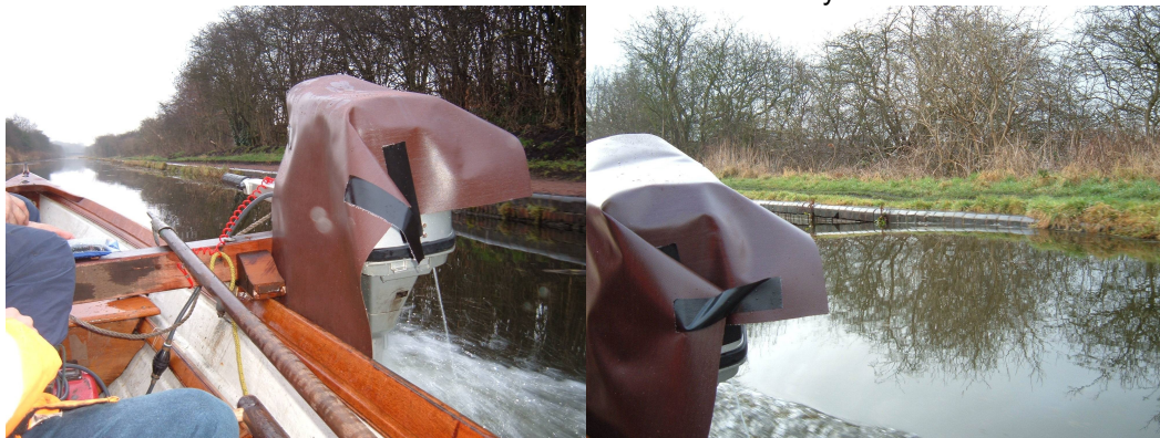
Whilst the engine created significant wash, the smooth soliton created by the boat can be seen well ahead. It arose shortly after the boat achieved the correct speed.
